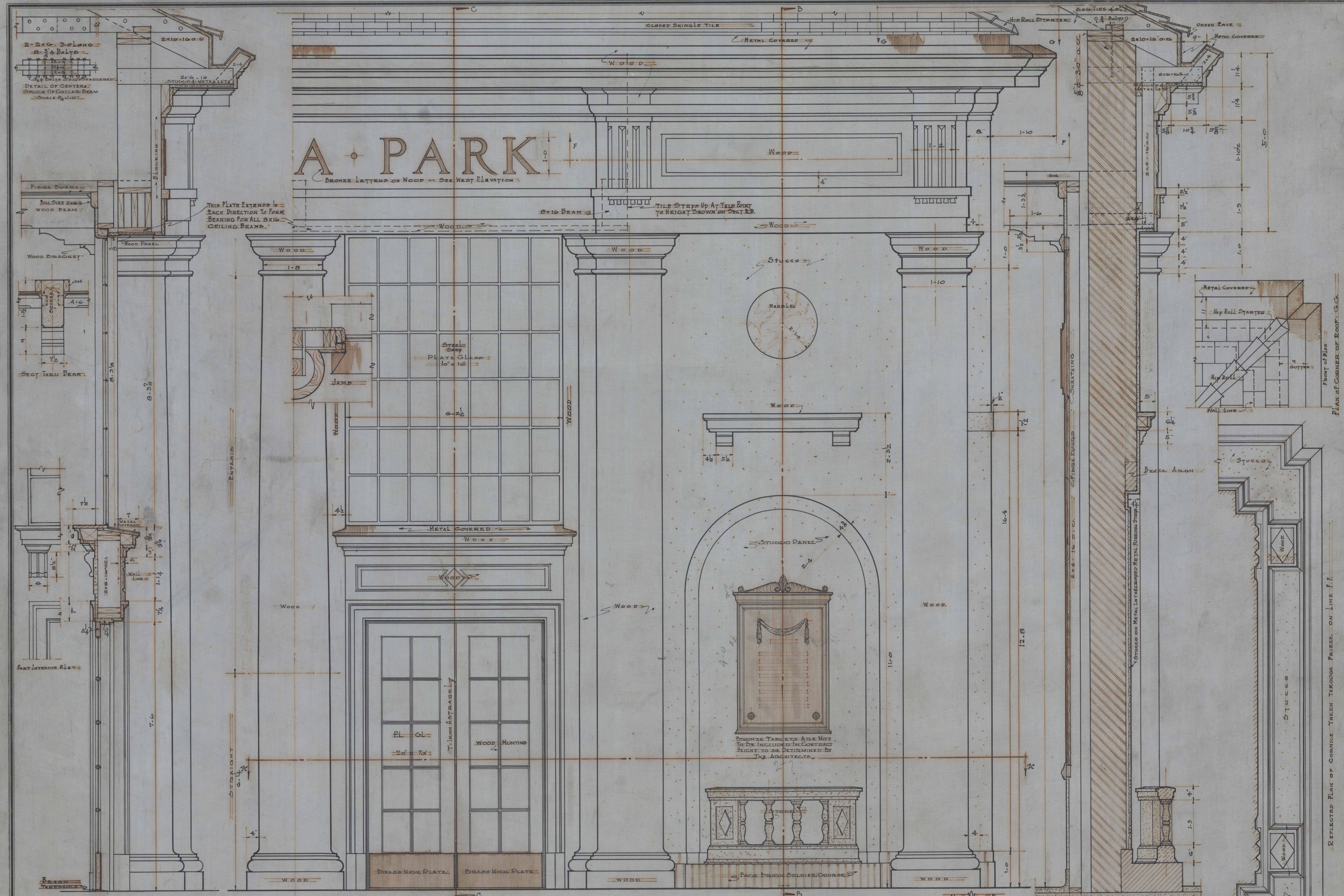
SECTION THIRD OF FRONT DOORS - SECTION C-C - SCALE 2 1/2" = 1'-0"
